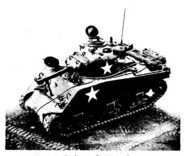
Figure 1. Medium tank, 105-mm howitzer.
