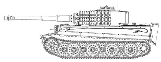
**Figure 13.** The **Tiger I**. This is officially *PzKpfw VI Ausf. H*. This version was the result of a competition of prototypes designed by Henschel and Krupp; the "H" indicates Henschel. The Krupp/Porsche consortium produced a number of chassis for their tank that were converted to heavily armored guns (the
