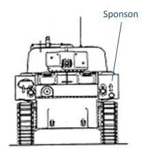
The armor on the M4 series was adequate. The first model had cast hull and cast turret, which improved integrity; some later models had welded plate hulls, some models reinforced (example being extra plates welded on the flanks to provide extra protection for ammunition storage).
