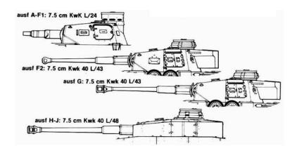
**Figure 12. Evolution of the PzKpfw IV**. The Pz IV was the heaviest tank in Germany's fleet in 1940, and began its active combat with a short 75mm L24 That eventually grew to an L48. There was a drive to add appliqué and bolt-on armor plates as well.
