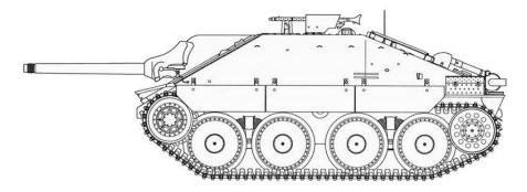
**Figure 14.** Hetzer (*Jagdpanzer* 38(t). This is a typical and numerous example of vehicle reuse. The Hetzer began life as a Czech tank mass produced by the Skoda Works. When Czechoslovakia joined the Reich, the model 38 (the (t) stands for "tschechisch") became the German Army's Pz 38(t). When it became obsolete, many chassis were converted to other uses, including this tank destroyer. The PzKpfw III and especially the IV were also converted to special combat functions.
