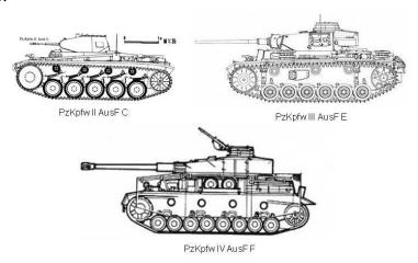
**Figure 11. Basic German tank thread**. The PzKpfw II, at less than 9 tons and armed with a 20mm gun, was by1943 reduced to a light reconnaissance role as the *Luchs* (Lynx). The PzKpfw III, which weighed in at 23 tons with a 37mm gun, was rarely seen in the East and reduced to a backup role elsewhere. The PzKpfw IV in various modifications lasted the entire war.
